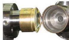
Figure 6. (a) Cup tool grinding
