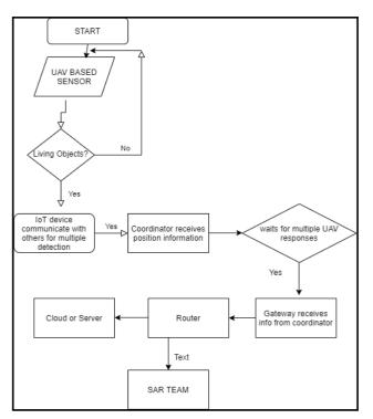
Fig. 3. Flow Chart of proposed Model's Working Principle
