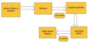
At first motion is detected by PIR sensor then it send the signal to Arduino Uno after that work is progressed as per code .This device take a step forward to home automation. This device will take a big role in corporate office, ATM, Bank vault which we discussed in future scope.
