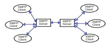
Fig. 6. Architecture of XMPP[19]
