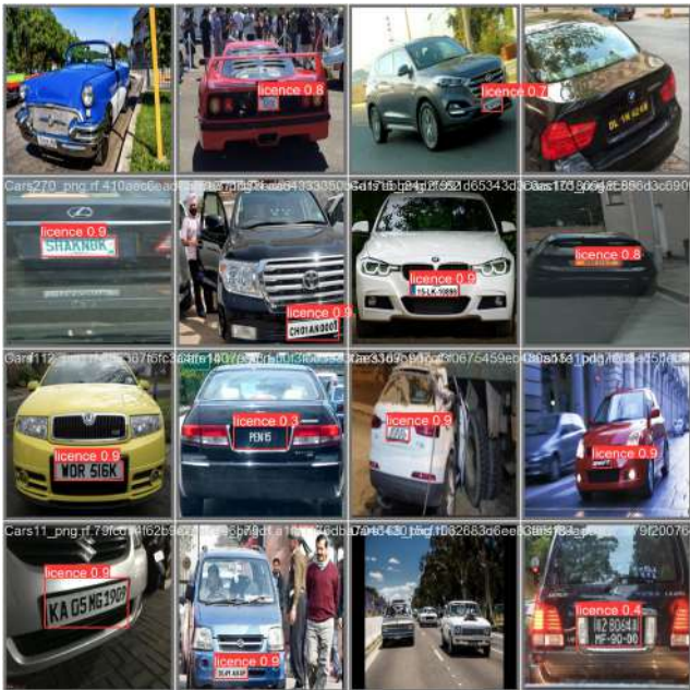
Fig:Plates identified by Yolov8
