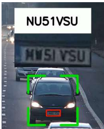
Fig:Licence text detection using EasyOcr
